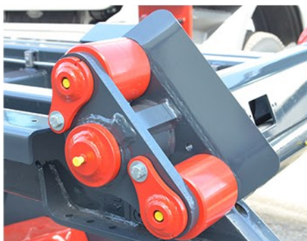
↳ Tandem rear rollers (option for DHT 40 and above)
