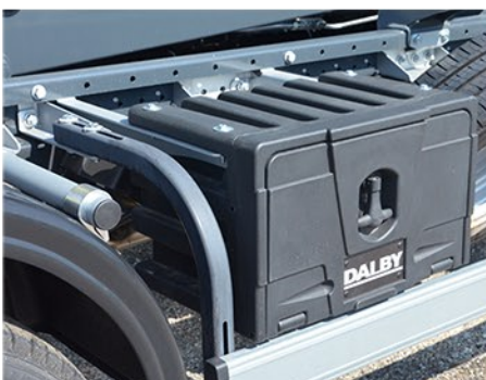
↳ Accessories bolted to the chassis
