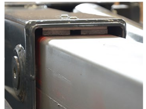
↳ Adjustable teflon sliding pads
